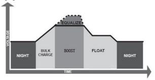
Figura4-2 eTracer-BND charging algorithm
