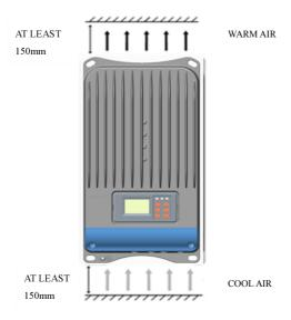
Figure3-1 Required mounting clearance for air
